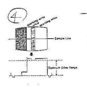
IF THE SIGNAL SURPASSES THE UPPER LIMIT, OR THE ELECTRIC CURRENT OF THE BEAM) IS TOO LARGE, IT CAUSES "BLOOMING," AND THE PICTURE IN THE BRIGHT AREA BECOMES BLURRED. OR, IF THE SIGNAL IS LESS THAN THE LOWER LIMIT, NO DETAILS WILL BE VISIBLE BECAUSE DARKER TONES CANNOT BE REPRODUCED ON THE SCREEN IN THIS RANGE.
